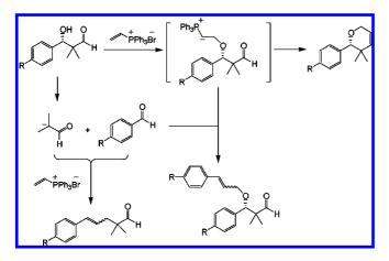
Exploring this reaction further led to an analogous tandem sequence, which consists of a conjugative addition, followed by an intramolecular cyclization/epoxidation process to afford 4,5-epoxytetrahydropyrans
